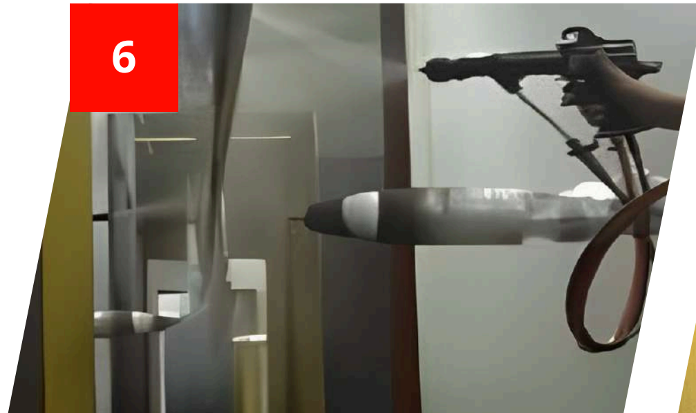
Wet Paint - Top Coat
